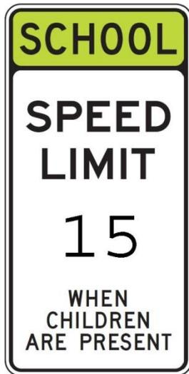
Figure 2 - School Speed Limit Sign is used to alert drivers to a change in the speed limit within the school zone area. In Wisconsin, the fixed speed limit for school zones is 15 MPH.
