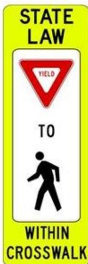
Figure 4 - In-Street School Crossing Sign is used as additional warning to drivers to indicate a crosswalk within a school zone.
